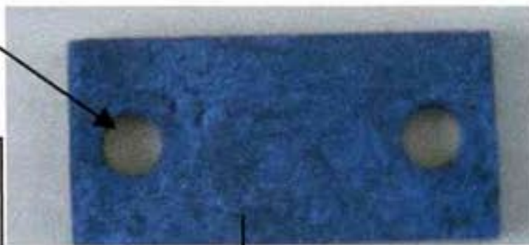
CC No.4 after removing products from the surface.Surface roughness was detected .Seven monts of exposure
