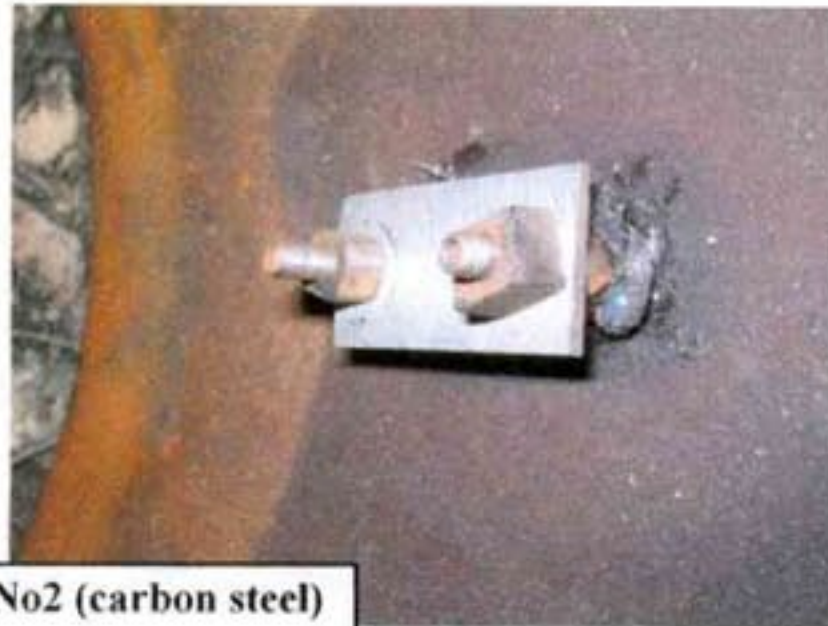
Fig.(7): Shows the installation of the Corrosion Coupon and Scale Coupon in Position No.4 (12inch)
