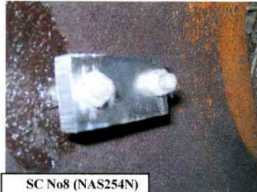
Fig.(7): Shows the installation of the Corrosion Coupon and Scale Coupon in Position No.4 (12inch)
