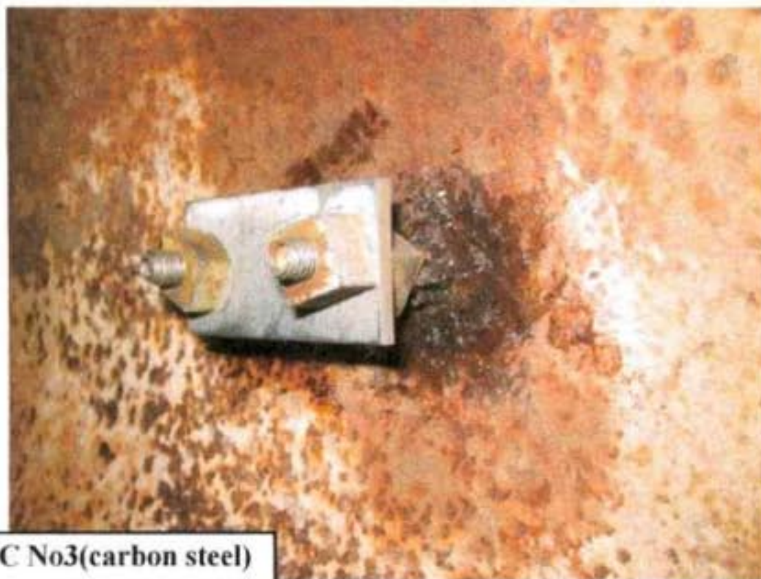
Fig.(6): Shows the installation of the Corrosion Coupon and Scale Coupon in Position No.3(10 inch)
