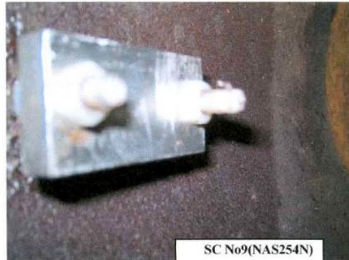
Fig.(6): Shows the installation of the Corrosion Coupon and Scale Coupon in Position No.3(10 inch)
